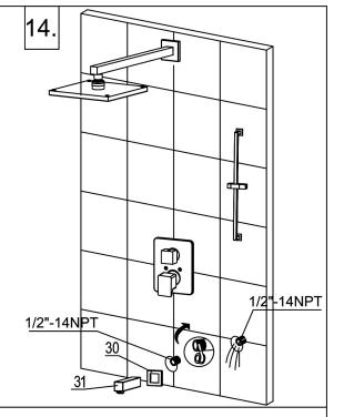
Tape the connector on the wall to install the decorative cover C (30) and spout (31).
