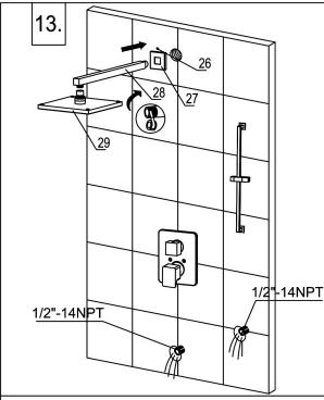
Use thread seal tape to tape the shower arm (28) as shown above. Assemble the decorative cover B (27), shower arm (28), and rainhead (29). Install it on the wall.
